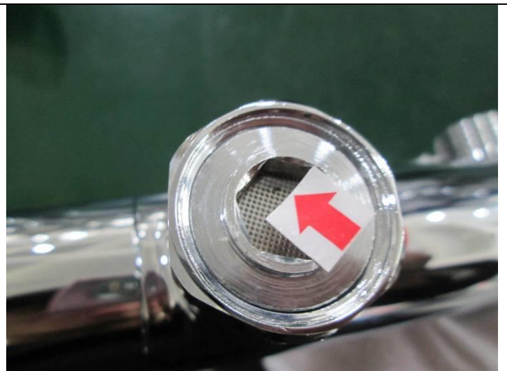
Rubbish inside side aerator - MIN
