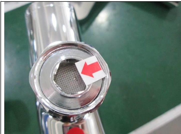
Rubbish inside side aerator - MIN
